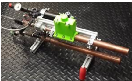
Figure 1 Prototype intelligent gas gun with magazine to hold 3 sensor packages.
