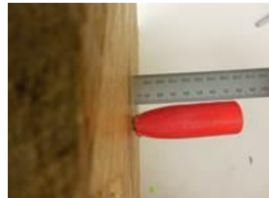
Figure 2. Remote sensor placement package embedded in a piece of fiber board using the remote sensor placement device.
